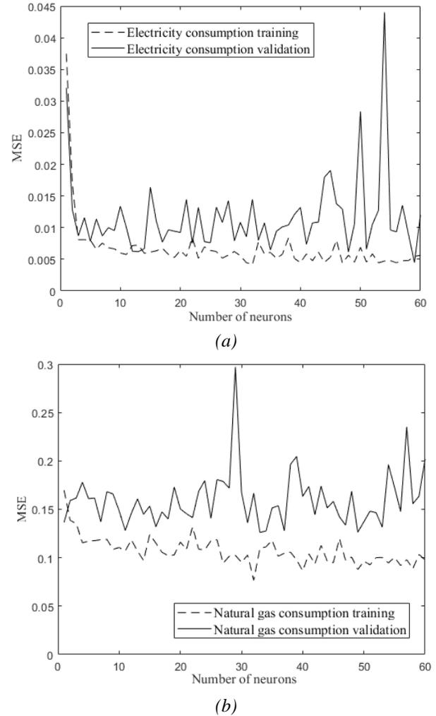
Figure 3. Results of sensitivity analysis of ANN model. (a) Electricity and (b) Natural gas consumption.
