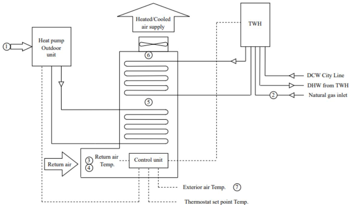
Figure 1. Schematics of the hybrid heating system and monitor measurements.
