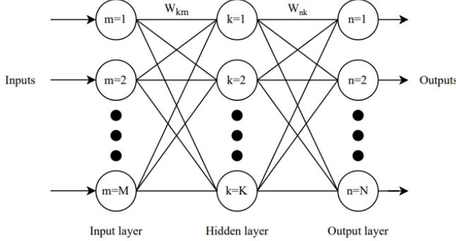
Figure 2. The structure artificial neural network (ANN).
