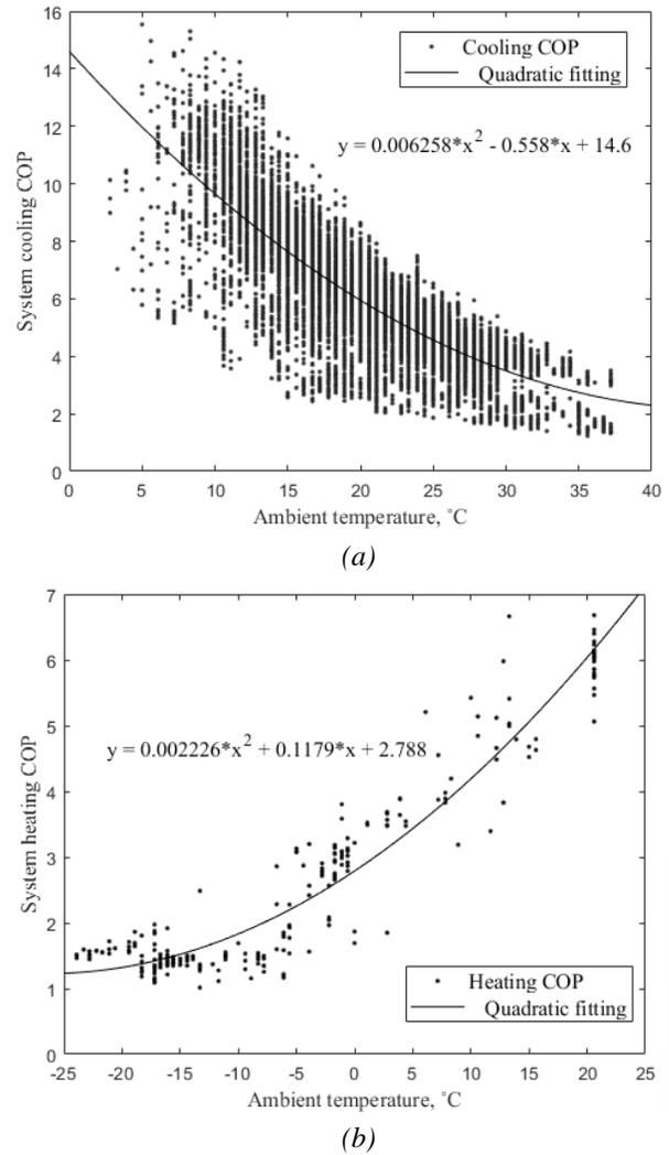
Figure 4. System (a)cooling COP and (b)heating COP operating heat pump under various ambient temperature.
