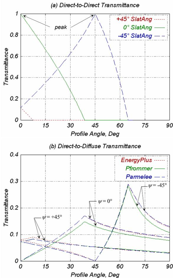
Figure 2 Effect of Slat Angle (for Flat Slat with Zero Thickness, and Slat Reflectance of 0.5): (a) Direct-to-Direct Transmittance, (b) Direct-to-Diffuse Transmittance
