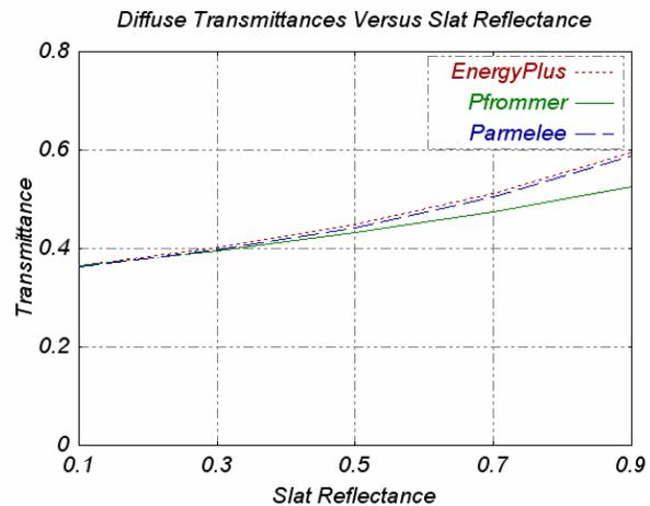
Figure 5 Effect of Slat Reflectance on Diffuse Transmittance(s) (for Flat Slat with Zero Thickness, and Slat Angle of  $0^\circ$ )
