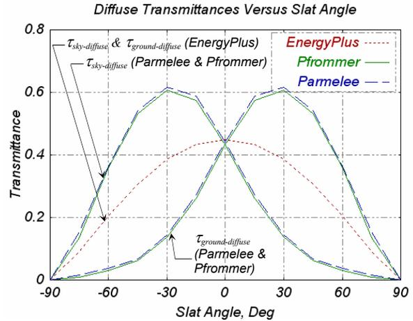
Figure 4 Effect of Slat Angle on Diffuse Transmittance(s) (for Flat Slat with Zero Thickness, and Slat Reflectance of 0.5)
