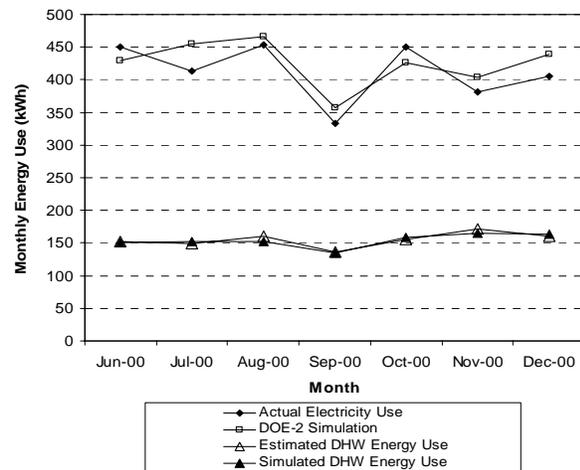
Figure 3: Comparison between the Actual and the Calibrated Simulated Electricity Use, including the Domestic Hot Water Energy Use from June to December, 2000.
