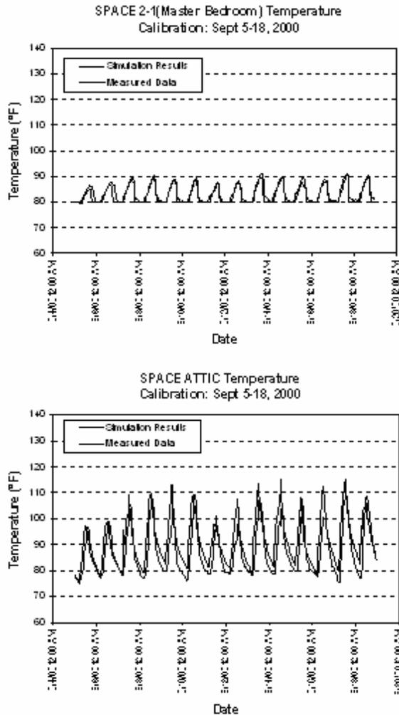
Figure 5: Comparison Between the Measured and the Calibrated Simulated Temperatures of the Master Bedroom (A/C was operated only in the nighttime (from 7:00 p.m. to 7:00 a.m.) and the Attic.
