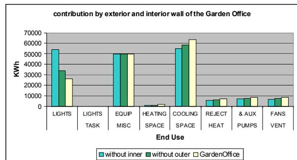
Fig 16: Contribution of the exterior and the interior walls against the total electric consumption. (using DOE 2 eQUEST)
