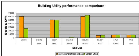
Fig 12 :Graph showing the difference in the performance of a Garden office to a conventional office building for different enduses. (using DOE 2 eQuest)
