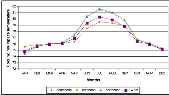
Fig 9 : Varying temperatures in a conventional office building for the various zones.
