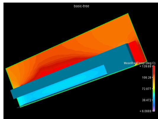
Fig 10 a.: Showing the MRT differential because of the raised floor
