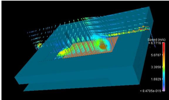
Fig 10 b.: The air movement caused due to the courtyard. (using Flovent, CFD)
