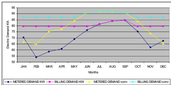
Fig 13: Graph demonstrating the difference in the Metered and Billing demand in KW for a Garden and a Conventional Office building.
