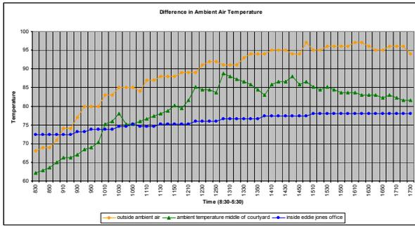
Fig3: Graph showing the difference in dry bulb temperature of Ambient Air :\_On the outside, within the courtyard and the inside of the case study building using measured data.
