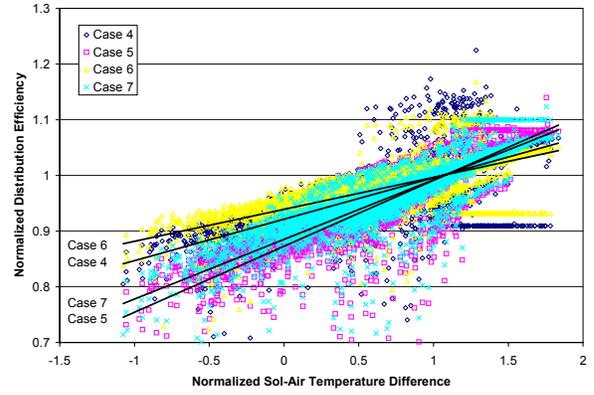
Figure 2 Distribution Efficiency Without Radiant Barrier, Heating
