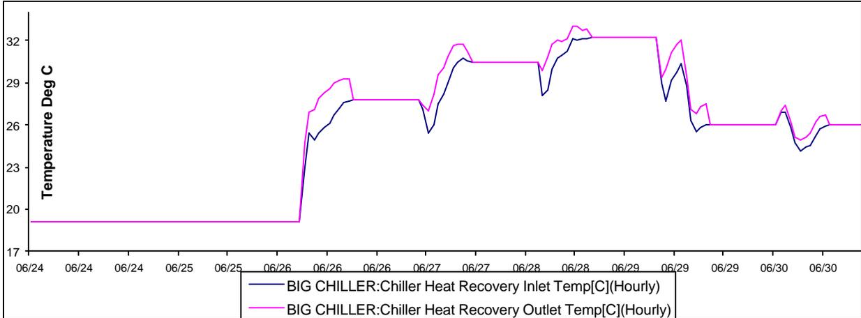
Figure 5: Heat Recovery Inlet and Outlet Temperatures
