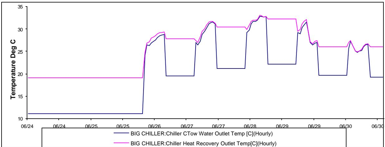
Figure 7: Outlet Heat Recovery & Outlet Chiller Condenser Temperature
