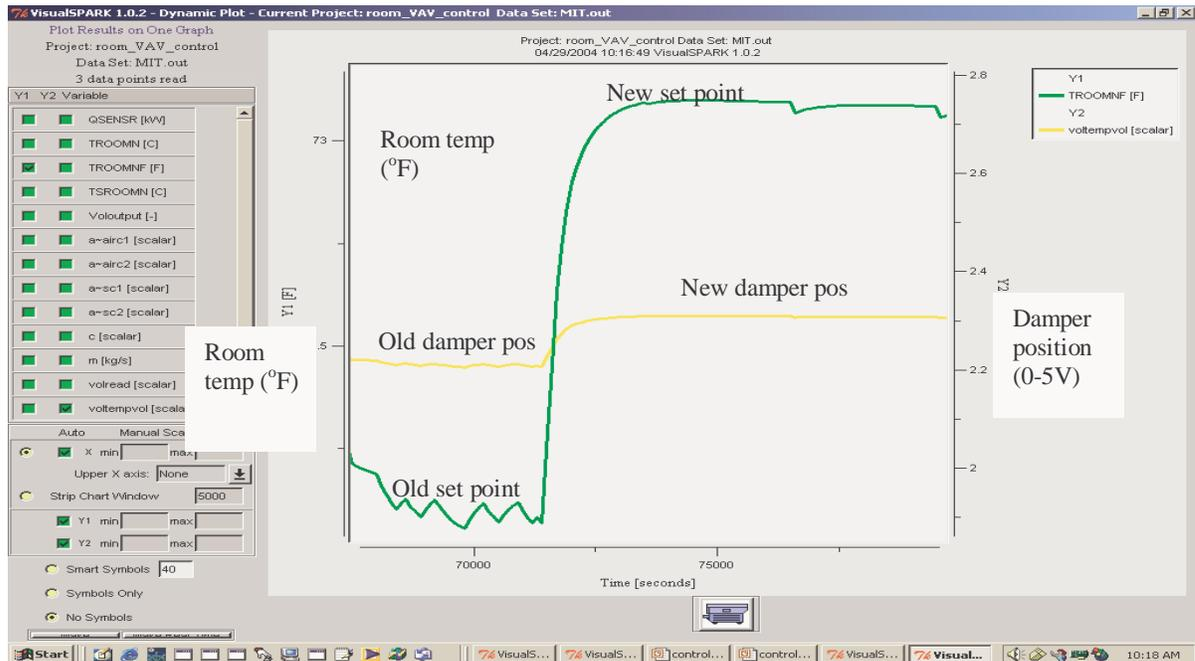
Figure 4 System response with tuned controller
