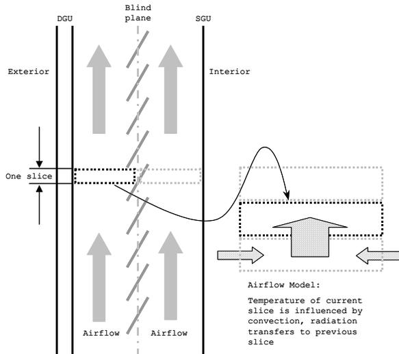
Figure 4. Iterative cavity air temperature calculation
