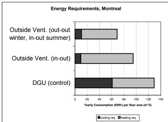
Figure 8. The outside-ventilated (in-out) typology gives the best overall result, but could be improved by adding the facility to switch the direction of the exhaust air, effectively turning the “in-out” window into an “out-out” window during certain months of the year
