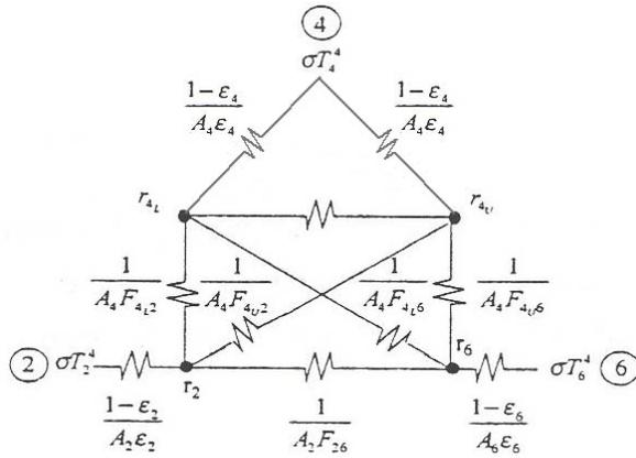
Figure 3. Resistive analogy for the 4-surface radiation problem (Illus. Dan Arons)
