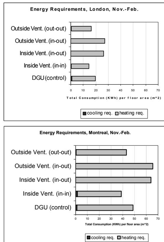
Figure 7. Heating and cooling loads for November through February only
