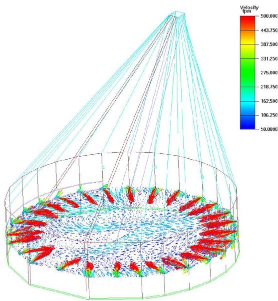
Figure 7 shows the flow at vent level as a vector plot. This macroscopic overview illustrates the general flow pattern inside the space at vent level.
