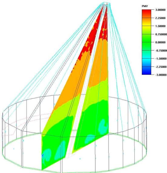
Figure 10 - Vertical Plane Cut For Predicted Mean Vote (PMV)
