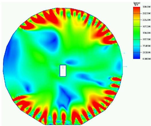
Figure 6 shows a horizontal plane cut for flow velocity at the height of the supply air vents. Supply vents are only placed around the perimeter of the occupied space and CFD was used to verify that fresh air would reach the center of the circular space. The analysis helped determine optimal vent placement, supply air volume, and vent type.
