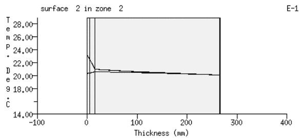
Figure 5. Temperature distribution through the PCM-composite wall
