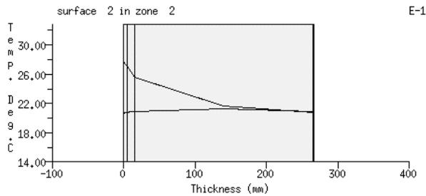
Figure 4. Temperature distribution through the ordinary ceramic wall
