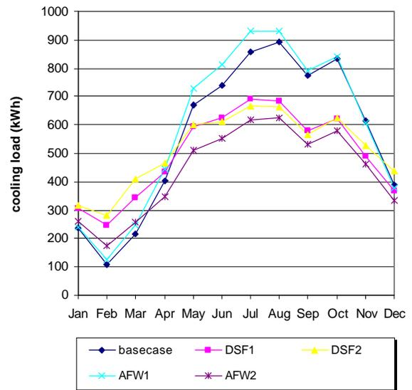
Figure 7. Simulation results for DSF and AFW
