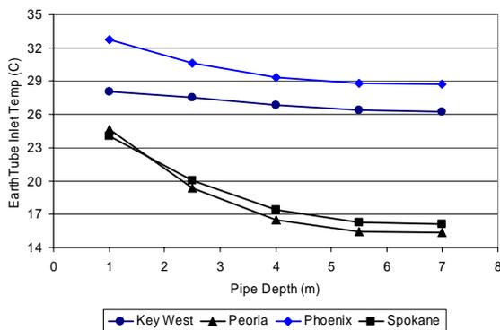
Figure 6. Influence of pipe depth on inlet temperature.
