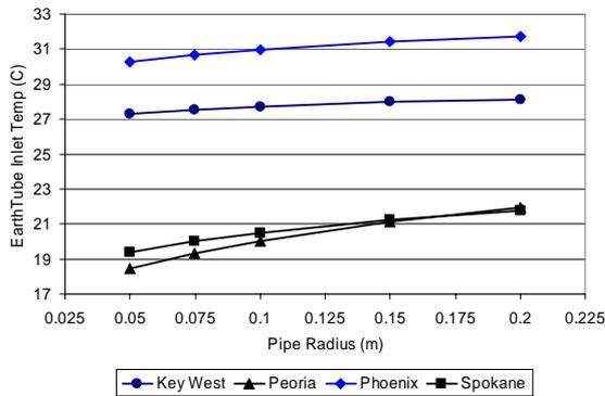
Figure 8. Influence of pipe radius on inlet temperature.
