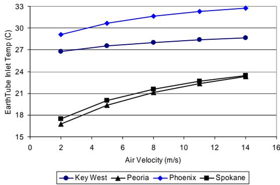
Figure 7. Influence of air velocity on inlet temperature.
