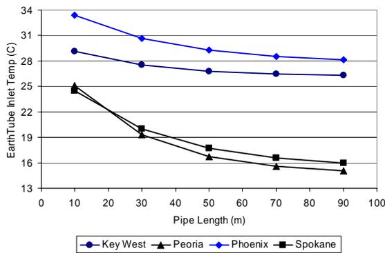
Figure 5. Influence of pipe length on inlet temperature.
