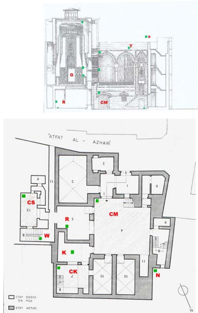
Figure 1 Ground Floor Plan & Section of the Case study House (Revault, 1997). Spaces: Main courtyard (CM), Service courtyard (CS), Kitchen courtyard (CK), Reception hall (R), summer hall (G), Rooftop solar Radiation shield (S). Note the places of the monitoring sensors in the main courtyard (CM), reception hall (R) & rooftop (S). Little square marks are the places of the sensors.
