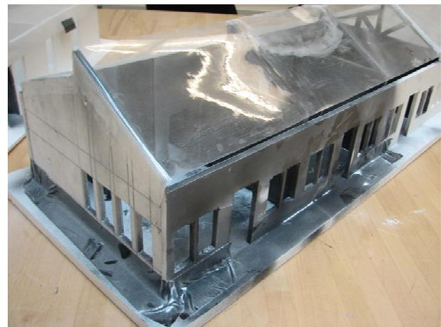
Figure 4. Airflow visualization and measurement model for the patient ward.
