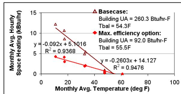
Figure 3: Determination of building UA and  $T_{bal}$
