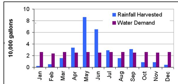
Figure 8: Rainwater supply and reduced water demand
