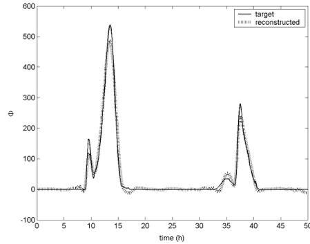
Figure 3: Incident solar radiation  $\Phi$ : target and reconstructed functions
