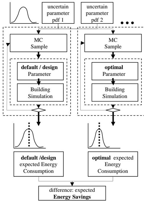
Figure 4: Flow chart for the determination of the expected energy savings from simultaneous optimization (right) and default design value MC simulations.
