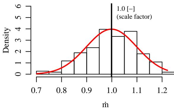
Figure 6: Distribution of the  $\dot{m}$  scaling parameter. Normal distribution with  $\mu=1.0$  and  $\sigma=0.20$ .
