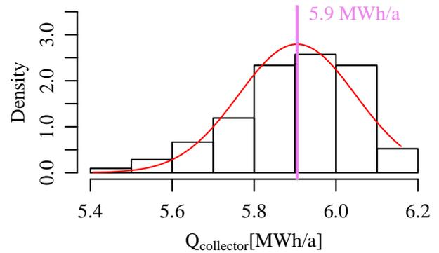
Figure 8: Distribution of the annual energy delivered by the collector system to the tank.
