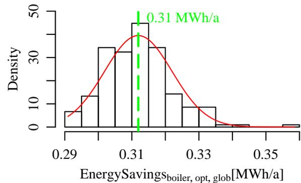
Figure 12: Distribution of the energy savings potential for the expectation of  $42.8^\circ$  of the optimal collector slope.
