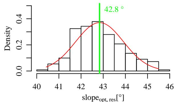
Figure 9: Distribution of optimal solar collector slope.
