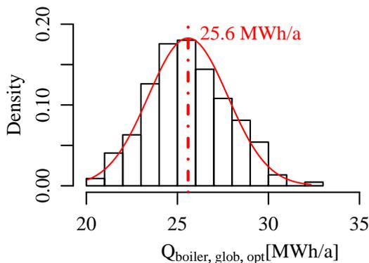
Figure 11: Distribution of the annual energy consumption of the boiler for the expectation of  $42.8^\circ$  of the optimal collector slope.
