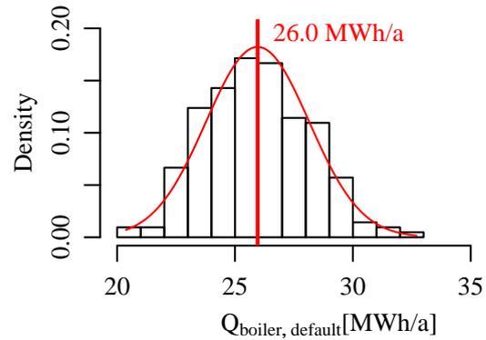
Figure 7: Distribution of the objective function: the annual energy consumption of the boiler.
