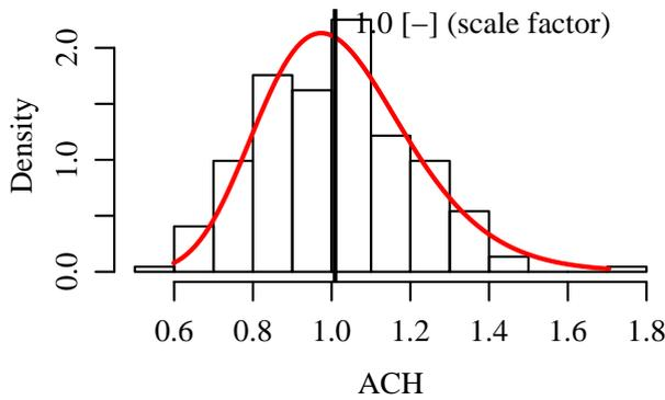
Figure 5: Distribution of the infiltration ACH scaling parameter. Log-normal distribution with  $\mu=1.0$  and  $\sigma=0.19$
