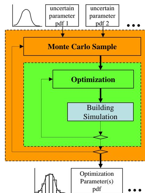
Figure 3: Flow chart of the optimization method.
