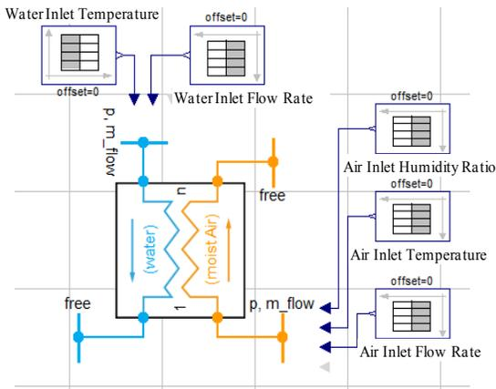
Figure 5: Dymola Layout for Evaporation Cooling Process of Cooling Tower
