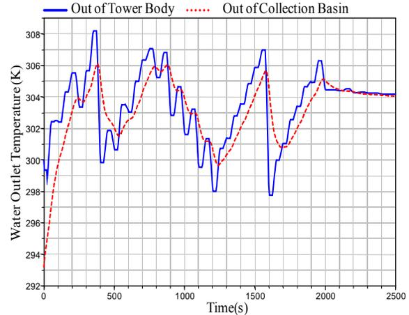
Figure 9: Transient Performance of Water Outlet Temperature - Comparison between Tower Body and Collection Basin Outputs
