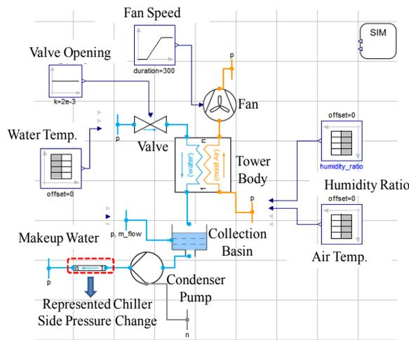
Figure 8: Dymola Layout for the Whole System of Cooling Tower Model
