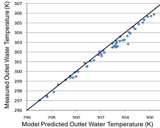
Figure 6: Comparison for Outlet Water Temperature between Model Prediction and Measured Data
