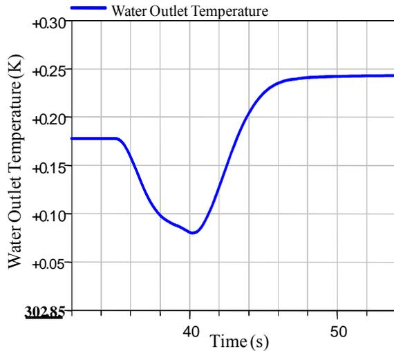
Figure 7: Transient Performance of Water Outlet Temperature - Stand-alone Cooling Tower Model
