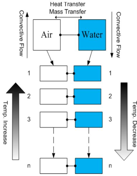
Figure 2: Illustration of Control Volumes for Cooling Tower Modeling
