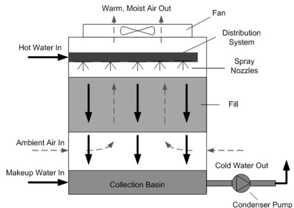
Figure 1: Schematic Diagram for Mechanical Draft Counter-Flow Wet Cooling Tower
