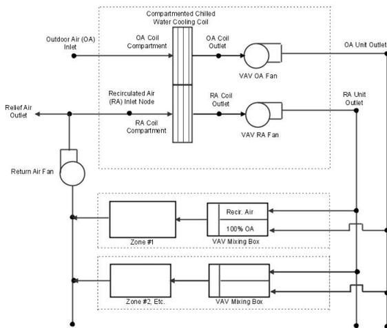
Figure 1 SCTF Airside System Topology
