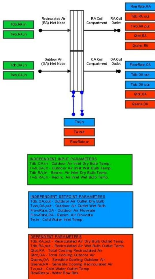
Figure 4 Compartmented Cooling Coil Diagram and Parameters
