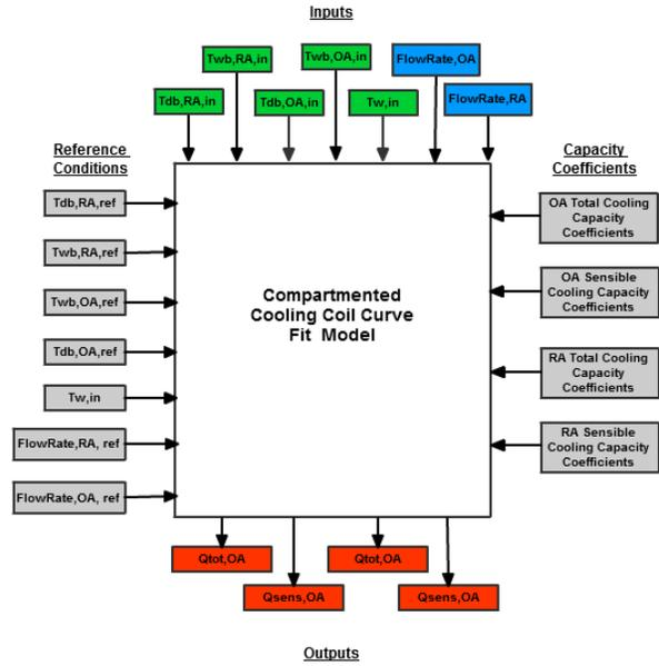
Figure 5 Compartmented Cooling Coil Curve Fit Model Information Flow
