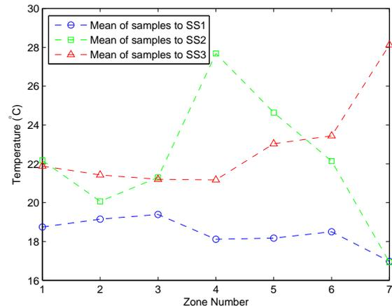
Figure 4: Mean initial zone temperatures for three different steady states
