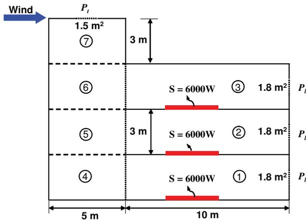
Figure 2: The geometries of the simulated building
