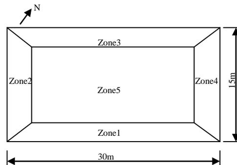
Figure 3 Geometry and horizontal zoning of the sample building
