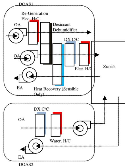
Figure 8 System configurations (CASE5)
