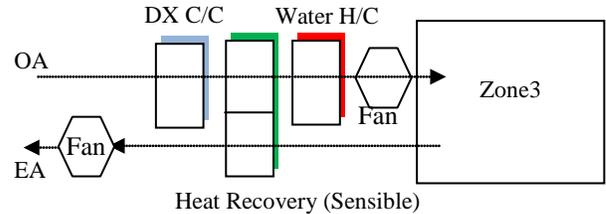
Figure 6 System configurations (CASE3)
