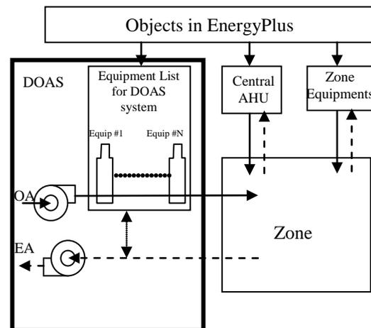
Figure 1 Diagram of a DOAS unit in EnergyPlus
