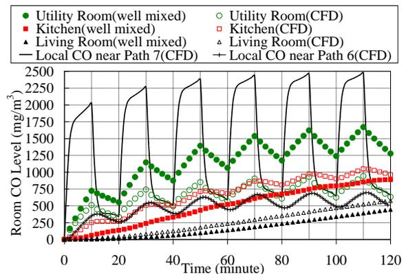
Figure 8 Comparison of CO levels in the utility room, kitchen, and living room of the house with and without CFD simulations
