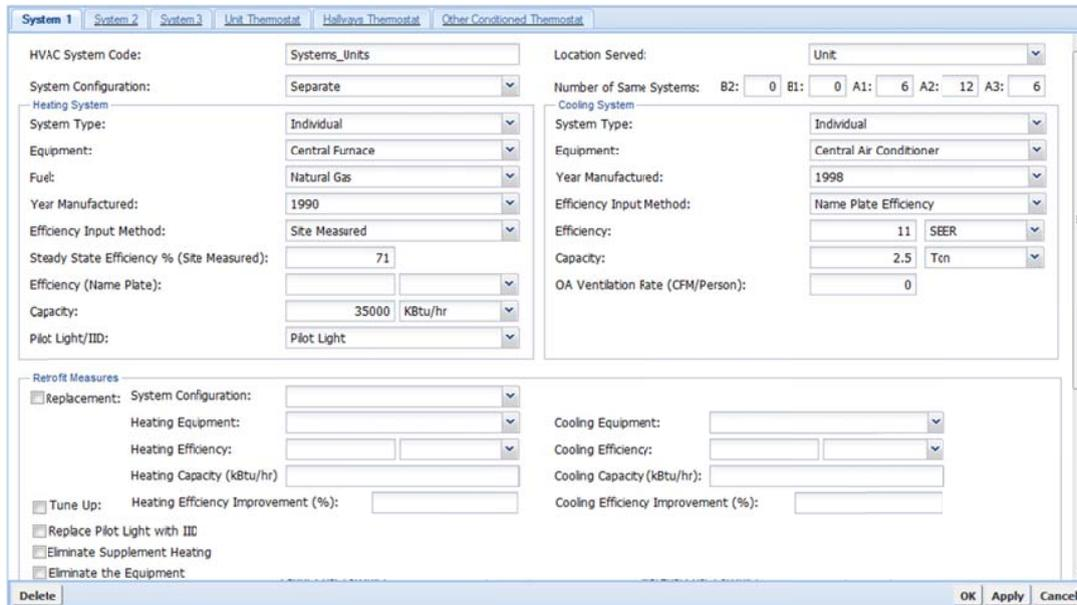
Figure 6: HVAC form for describing system type, size, efficiency, and retrofit measures
