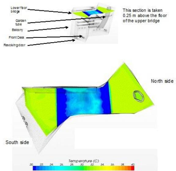
Figure 12 Temperature distribution in the middle of atrium
