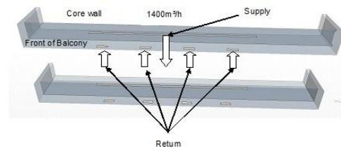
Figure 3 The balcony returns and supply outlets and their location
