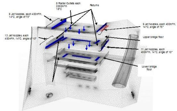
Figure 14 Variant 2 geometry
