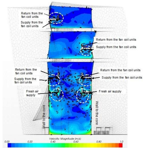
Figure 8 Velocity distribution through the balconies
