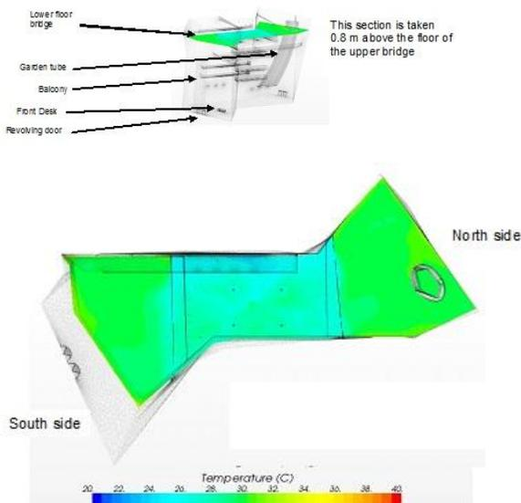
Figure 17 Temperature distribution in the middle of atrium
