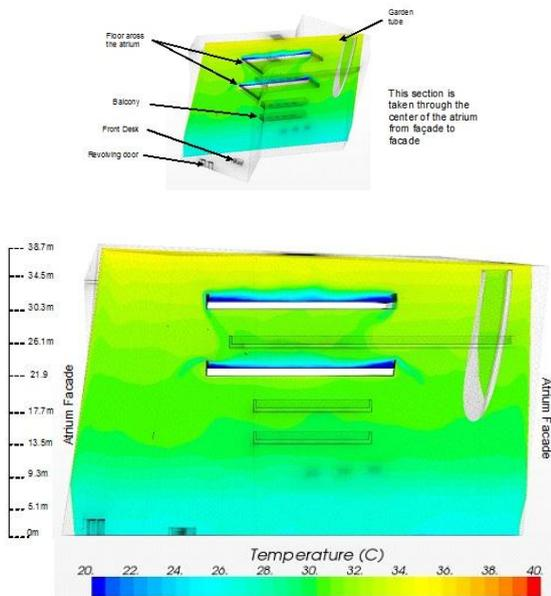
Figure 10 Temperature distribution in the middle of atrium
