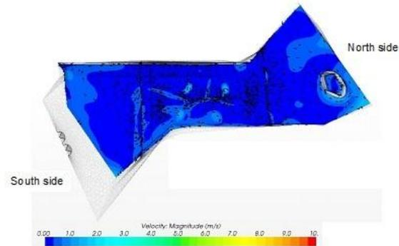
Figure 18 Velocity distribution in the middle of atrium
