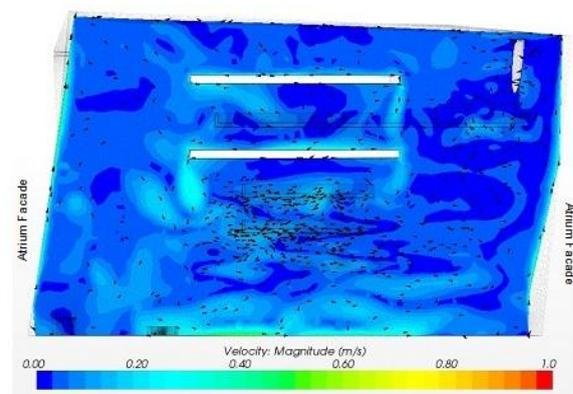
Figure 6 Velocity distribution in the middle of the atrium
