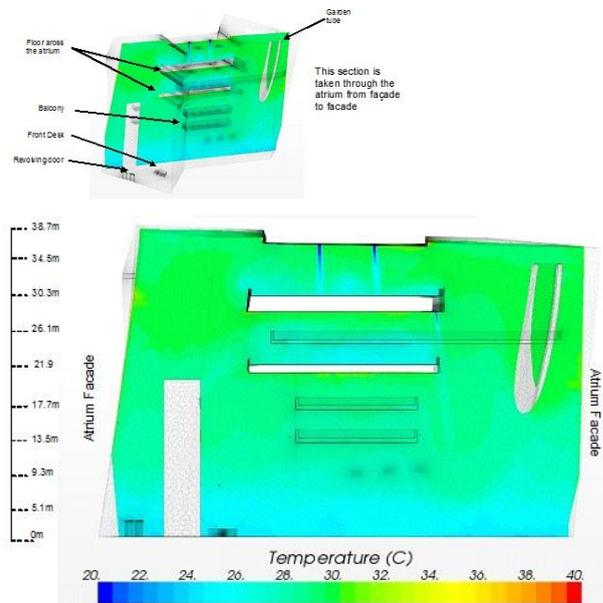
Figure 15 Temperature distribution in the middle of atrium
