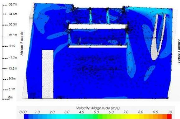
Figure 16 Velocity distribution in the middle of atrium
