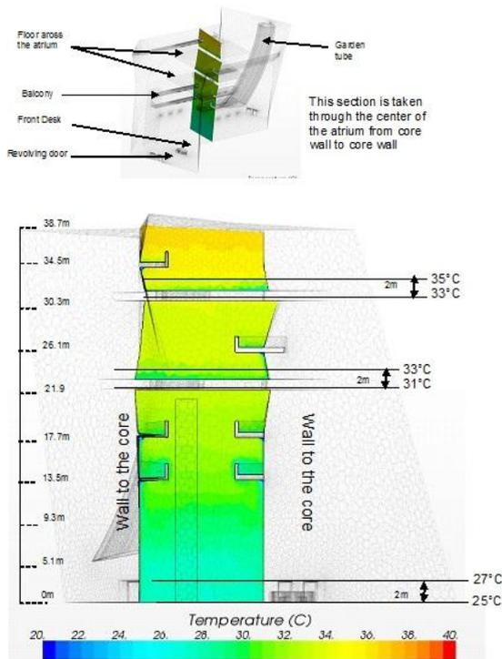
Figure 7 Temperature distribution through the balconies
