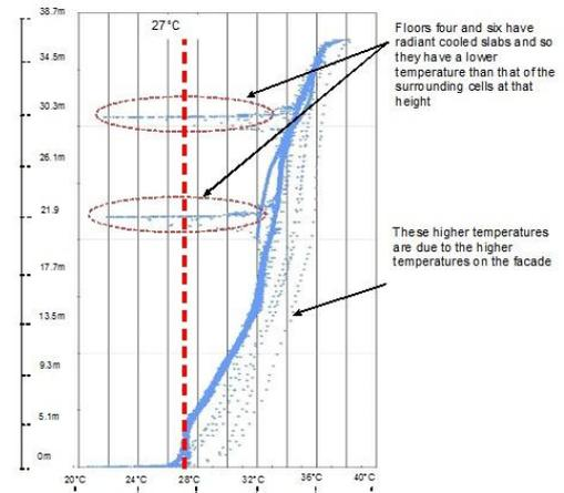
Figure 5 Temperature of the atrium at different heights
