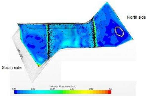
Figure 13 Velocity distribution in the middle of atrium
