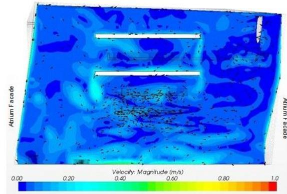
Figure 11 Velocity distribution in the middle of atrium
