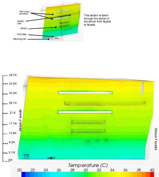
Figure 4 Temperature distribution in the middle of the atrium
