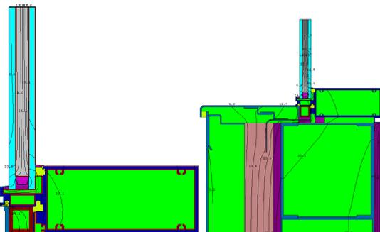
Figures 5 & 6. THERM models: A2-CL (left) and A2W2-CL (right).
