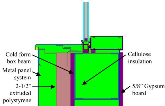
Figure 4. Model A2-CL showing wall construction.
