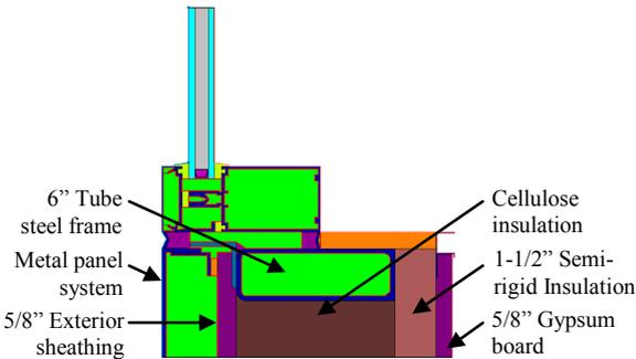
Figure 1. Model A1-CL showing wall construction.
