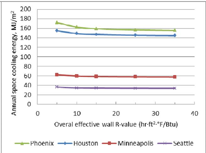
Figure 12 Effects of opaque wall thermal resistance on space cooling for medium office
