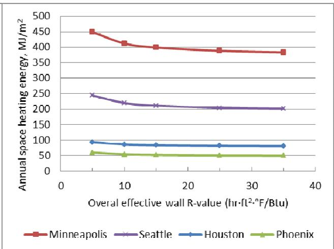
Figure 10 Effects of opaque wall thermal resistance on space heating for a midrise MURB with 60% glazing
