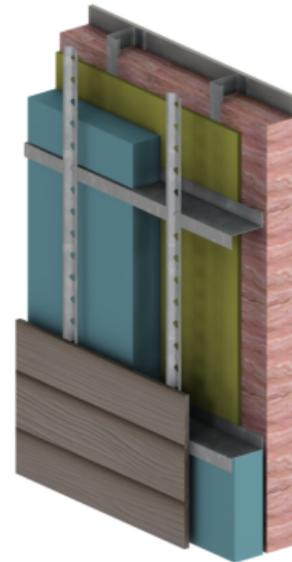
*Figure 6 R-20 exterior and R-13 interior split insulated steel stud assembly with horizontal z-girts*
