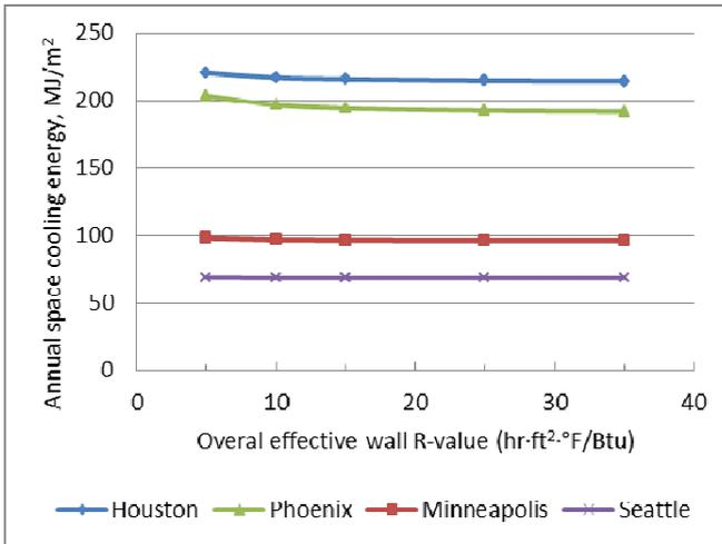
Figure 11 Effects of opaque wall thermal resistance on space cooling for a large office
