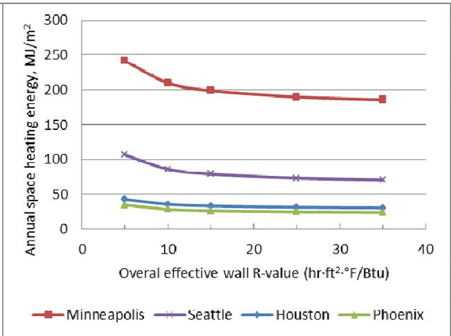
Figure 8 Effects of opaque wall thermal resistance on space heating for medium office
