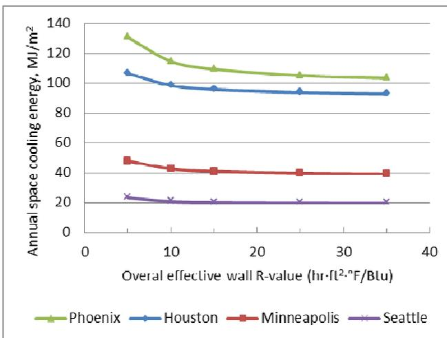
Figure 13 Effects of opaque wall thermal resistance on space cooling for midrise MURB with 15% glazing
