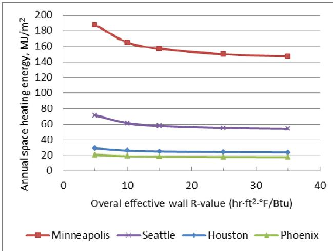
Figure 7 Effects of opaque wall thermal resistance on space heating for a large office
