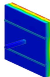
Figure 5 Example point transmittance detail
