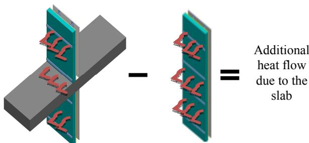
Figure 2 Determining linear transmittance for a slab
