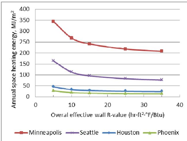
Figure 9 Effects of opaque wall thermal resistance on space heating for midrise MURB with 15% glazing
