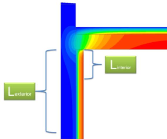
Figure 1 Effective lengths for area-weighted calculations for parapet from exterior and interior
