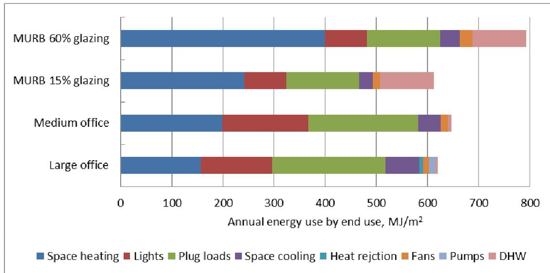
Figure 15 Annual building energy by end use for various building types in Minneapolis with an effective wall thermal resistance of R-15
