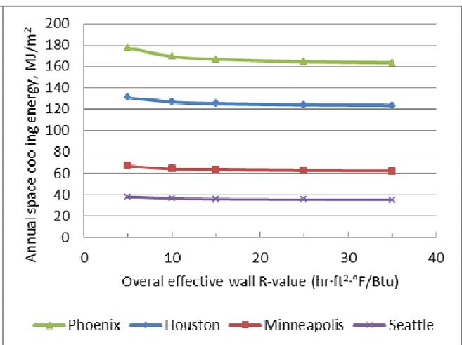
Figure 14 Effects of opaque wall thermal resistance on space cooling for a midrise MURB with 60% glazing
