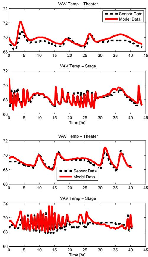
Figure 5: Dynamic Response of the Zone Temperatures in the Theater and Sound Stage for the Calibrated Model Compared to Sensor Data (two different cases).
