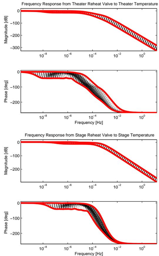
Figure 6: Bode response for the reheat function of both the theater and sound stage. Three hundred realizations of different parameter combinations captures the uncertainty in the identified model. The solid lines illustrate the boundary of the uncertain set of the frequency response.
