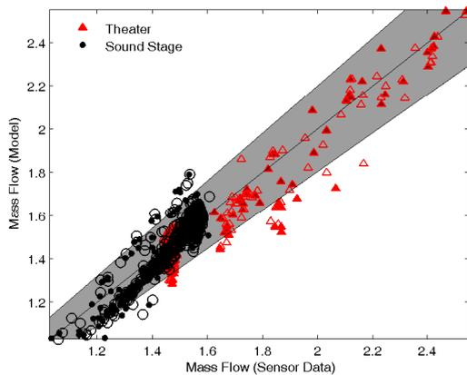
Figure 4: Calibration of the steady state flow network including the fan. The solid markers are calibration data and the empty markers are verification data. The grey area identifies the bounds of 10% error.
