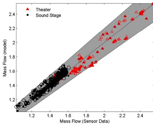
Figure 3: Calibration of the steady state flow network, the solid markers are calibration data and the empty markers are verification data. The grey area identifies the bounds of 10% error.
