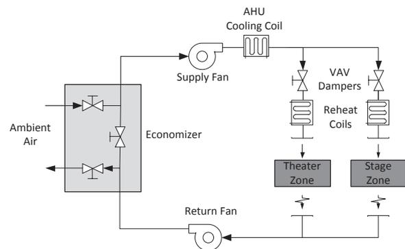
Figure 2: Schematic of the heating and cooling equipment in the Theater.
