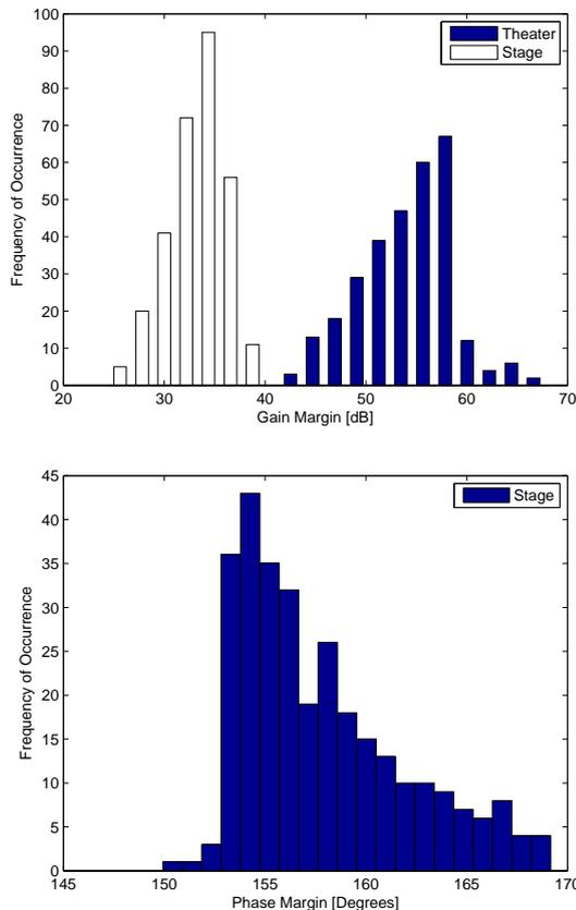
Figure 7: Gain and phase margins for the reheat control. Three hundred realizations of different parameter combinations captures the uncertainty in the identified model. The phase margin for the theater is infinite within the bounds of uncertainty in parameters.
