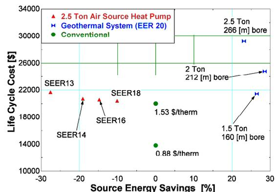
Figure 2: Heat pump systems vs. the conventional system (at two different natural gas rates) in the Chicago location. The fuel inflation rate in this analysis is 15%.
