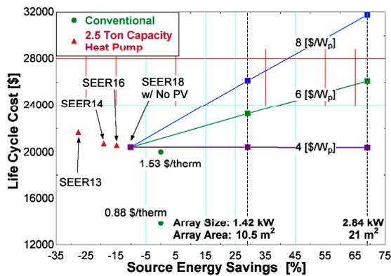
Figure 5: Heat pump system with PV vs. the conventional system in the Chicago location. The fuel inflation rate in this analysis is 15%.
