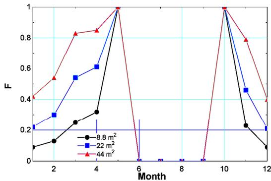
Figure 9: Fraction of the heating load met by the solar thermal system for each month.
