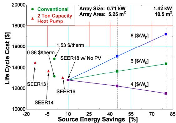
Figure 6: Heat pump system with PV vs. the conventional system in the Dallas location. The fuel inflation rate in this analysis is 15%.
