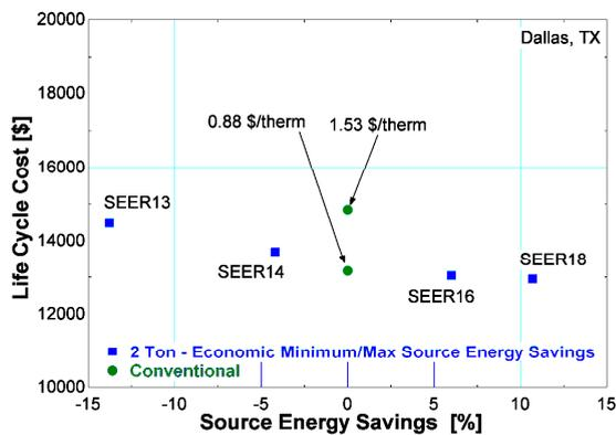
Figure 3: Heat pump system vs. the conventional system (at two different natural gas rates) in the Dallas location. The triangles represent the most source energy savings. The fuel inflation rate in this analysis is 15%.
