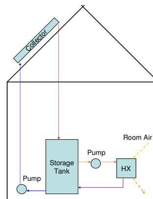
Figure 7: Solar thermal system model used for house heating. Water is the working fluid and a drain back system is used to prevent freezing.
