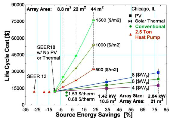
Figure 8: Solar thermal and PV results for the Chicago location. The fuel inflation rate for this simulation was 5%.
