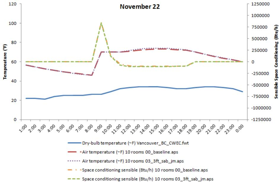
Figure 4 Peak Heating Day Hourly Analysis in Climate 5C
