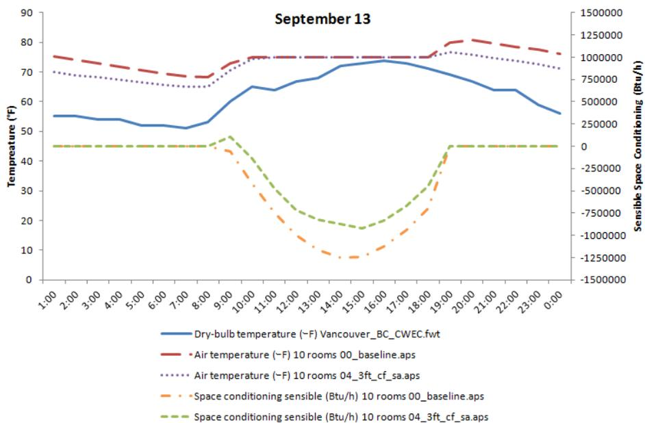
Figure 5 Peak Cooling Day Hourly Analysis in Climate 5C
