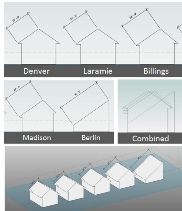
*Figure 9 Roof and Corresponding House Shapes Needed to Achieve Net-Zero by Location, by Autodesk Vasari*
