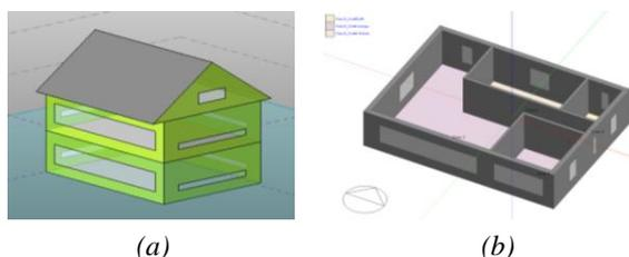
*Figure 7 Energy Simulation Models in (a) Vasari and (b) Design Builder.*
