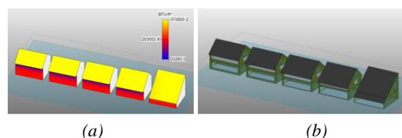
*Figure 10 NZE homes by location showing (a) annual solar radiation, (b) energy model with optimal south glazing ratios, by Autodesk Vasari*
