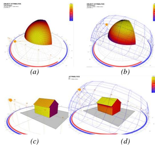
Figure 5 (a) Sphere Analysis Dec 07 – Jan 06; (b) Annual Sphere Analysis (c) Solar Radiation Analysis Dec 07 – Jan 06; (d) Annual Solar Radiation Analysis in Laramie, by Autodesk Ecotect.
