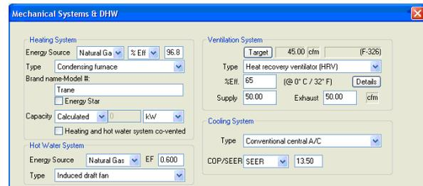
Figure 3. Data input for the mechanical systems.
