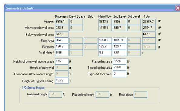
Figure 5. Checking and correcting geometry details.
