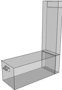
Figure 6: Schematic of Single Zone example case simulated in EnergyPlus and CFD. A pivoted inlet window is on the left of the room zone and at the far end is a stack exhaust with an outlet near the top.
