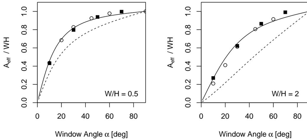
Figure 4: Effective area  $A_{eff}$  for top-pivoted windows scaled by  $WH$ , for (a) narrow window, and (b) wide window from the original (---) and modified (—) EnergyPlus parameterizations, CFD test results for the simple window (■), and measured data reported by IES MacroFlo (o).
