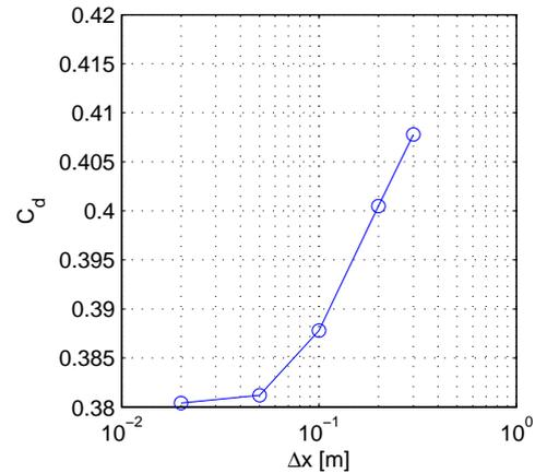
Figure 3: Effect of grid resolution on discharge coefficient. Here, the angle of the pivoted window is  $30^\circ$  and the flow rate is  $0.28\text{m}^3/\text{s}$  through the full window opening (1.2m long by 0.6m high).
