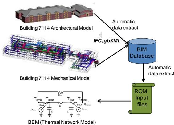
Figure 13 BIM to BEM Flow Chart
