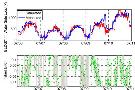
Figure 15 Building 7114 Real-Time Simulation Results from 07/06/2011 to 07/11/2011.
