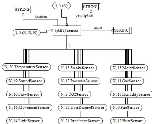
Figure 6 Sensor Schema
