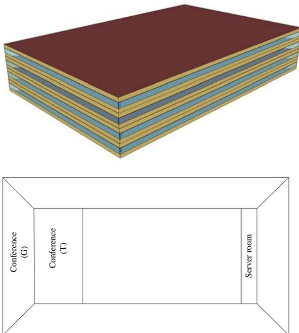
Figure 1: Axonometric view (top) and thermal zoning (bottom) of the large office building
