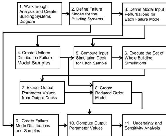
Figure 1: Overall process flow for analyzing effects of failure modes on building energy.
