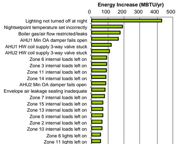
Figure 4: Sensitivity of Overall Building Energy Consumption to the top contributing Failure Modes.
