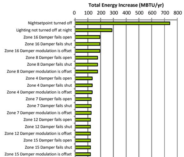
Figure 6: Sensitivity of Overall Building Energy Consumption to the top contributing Failure Modes.
