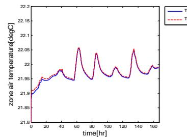
Figure 4: Comparison of dynamic zone air temperature behavior between full-order and reduced-order models
