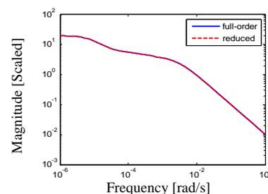
Figure 5: Frequency response of zone air temperature to mechanical cooling
