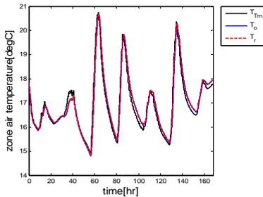
Figure 3: Model comparisons between TRNSYS, full-order, and reduced-order models
