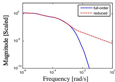
Figure 6: Frequency response of zone air temperature to solar disturbance
