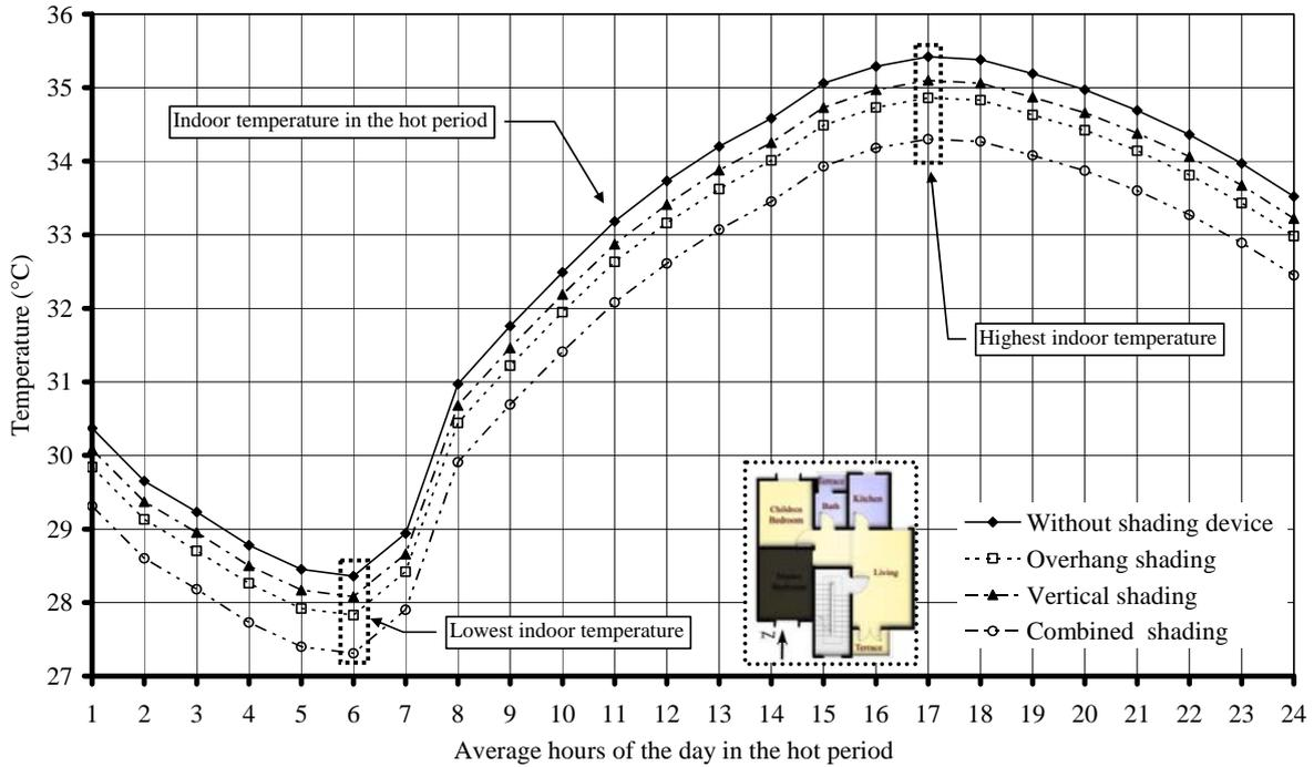
Fig 17 Values of indoor temperatures for the Southern oriented bedroom, for different shading devices types adjoining the room window – in the residential model (hot period)
