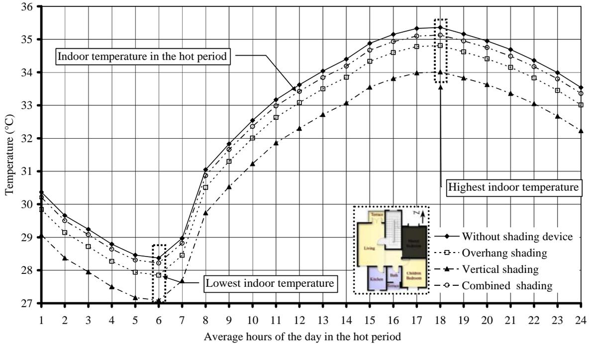
Fig 15 Values of indoor temperatures for the Northern oriented bedroom, for different shading devices types adjoining the room window – in the residential model (hot period)
