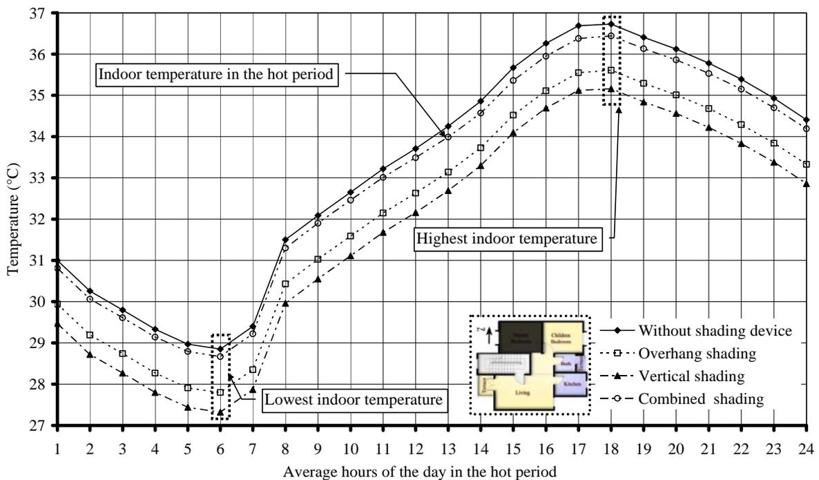
Fig 18 Values of indoor temperatures for the Western oriented bedroom, for different shading devices types adjoining the room window – in the residential model (hot period)
