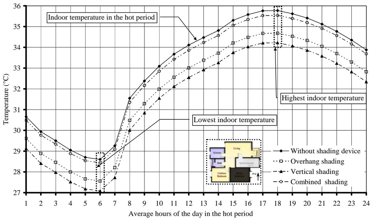
Fig 16 Values of indoor temperatures for the Eastern oriented bedroom, for different shading devices types adjoining the room window – in the residential model (hot period)
