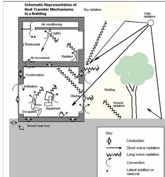
Fig 8 The influence of temperature on the outer envelop of the building and indoor.[6]
