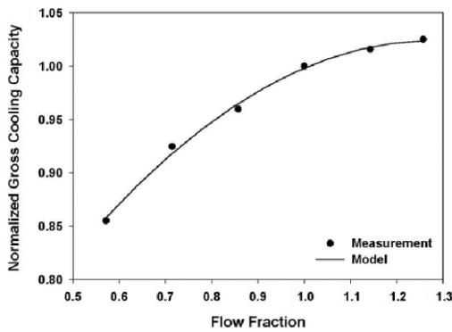
Figure 4 Normalized gross cooling capacity as a function of FF
