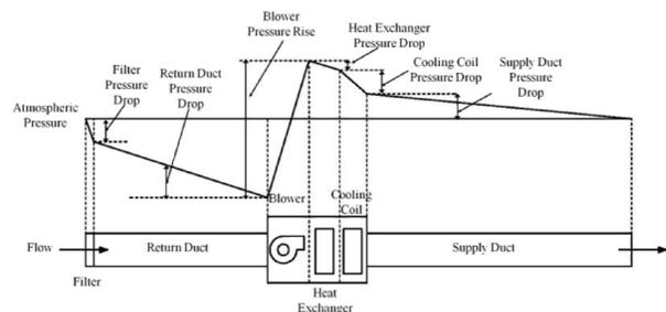
Figure 1 Theoretical static pressure changes for a typical residential system
