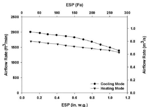
Figure 2 Airflow performance of the ECM blower
