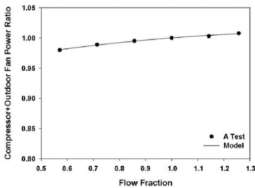
Figure 5. Normalized outdoor fan/compressor power draw as a function of FF
