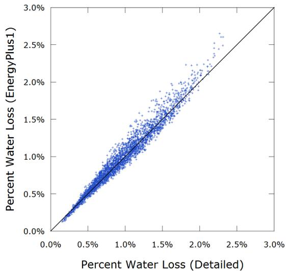
Figure 5 EnergyPlus1 vs detailed model
