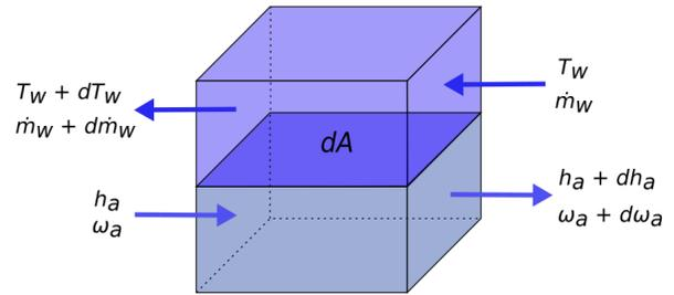
Figure 2 Differential tower element
