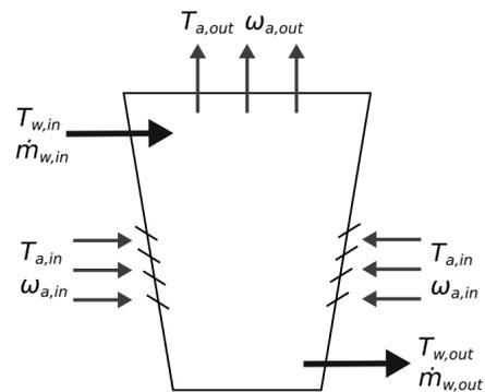
Figure 1 Cooling tower schematic
