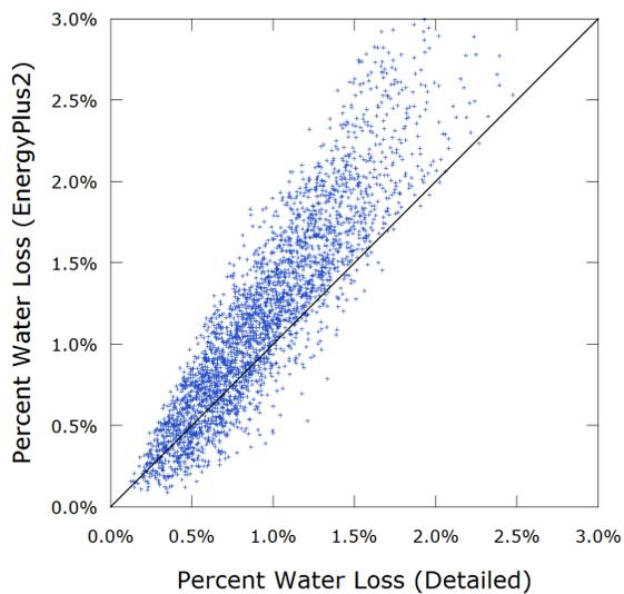
Figure 6 EnergyPlus2 vs detailed model
