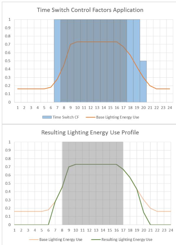
Figure 12: Application of Time Switch Control Factor for a space with 8:00am to 5:00pm operation schedule (grey) and 1.5 hour delay time on override switch
