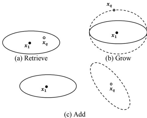
Figure 1. Three actions of ISAT algorithm.
