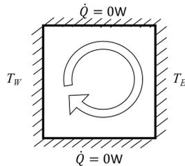
Figure 3 Schematic of the natural convection flow
