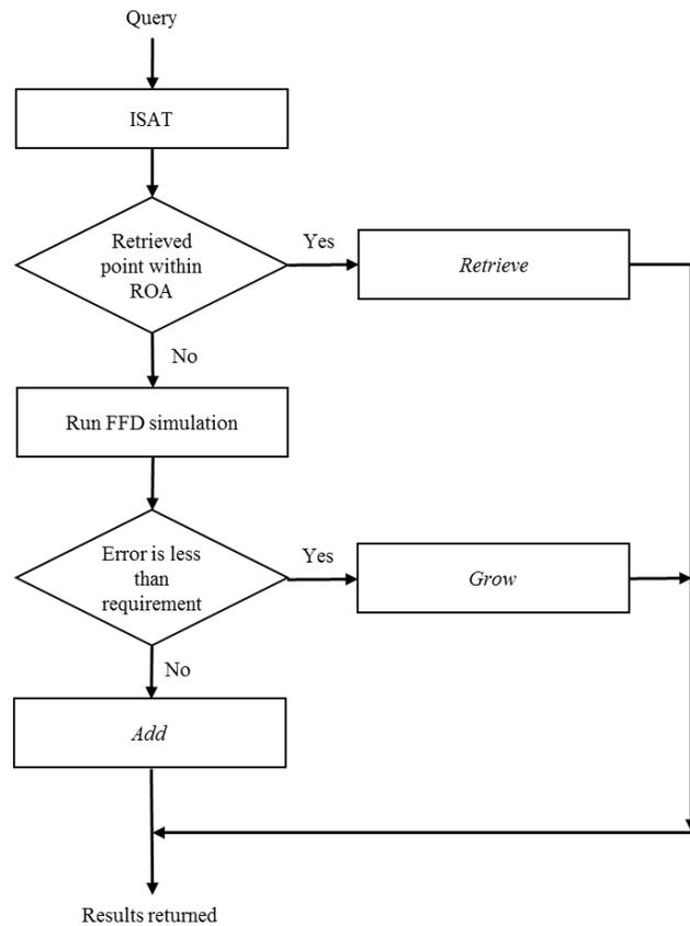
Figure 2. Workflow of the ISAT-FFD algorithm.
