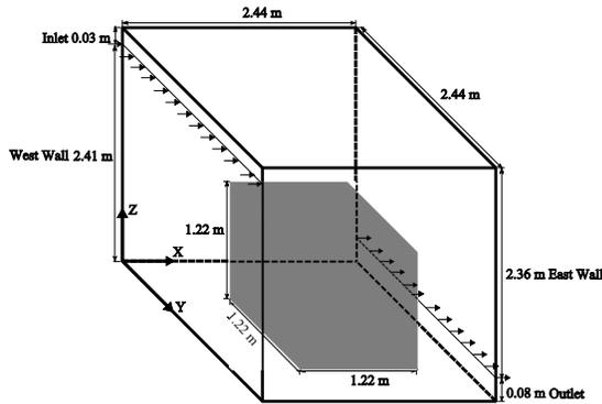
Figure 5 Schematic of the mixed convection in an empty room with a heated box
