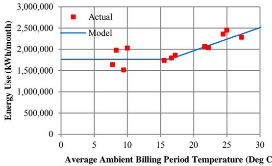
Figure 5. Actual Energy Usage vs 3PC Model Prediction for Facility B
