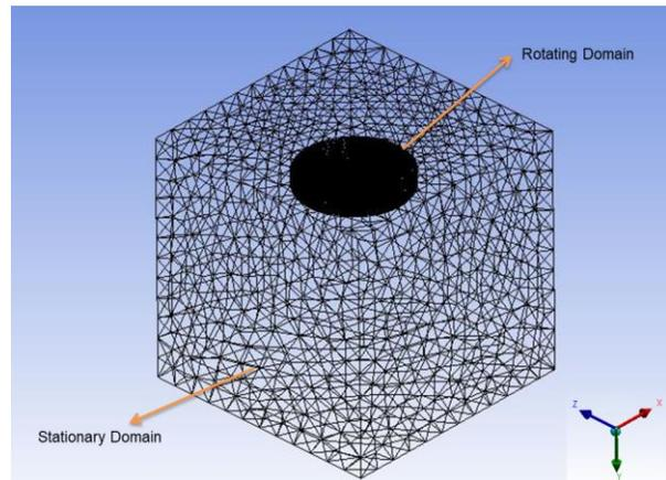
Figure 6 Computation domains of CFD model and grid structure
