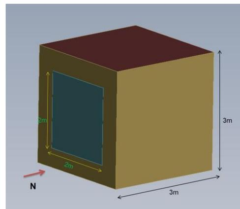
Figure 3 Computational domain for EnergyPlus model
