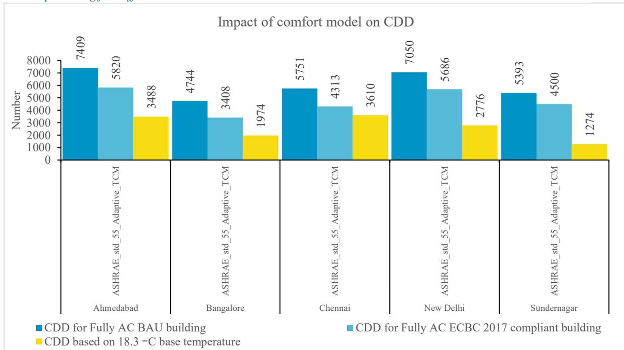
Figure 2: Impact of adaptive comfort model on CDD values
