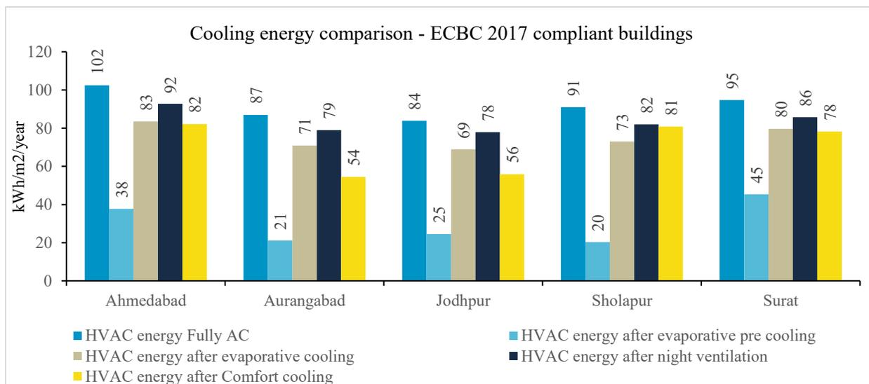
Figure 4: Annual cooling energy for ECBC 2017 compliant building after applying passive strategy
