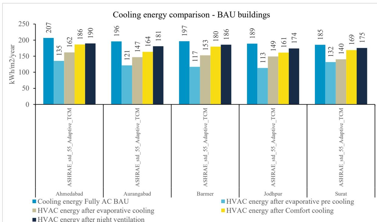
Figure 3: Annual cooling energy estimation of BAU buildings
