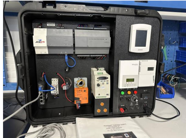
Figure 2. An example of the BAS simulator used for the iConnect training program equipped with sensors and controllers for hands-on experiences.
