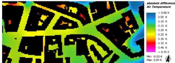
Figure 9: Temperature difference between Case 1 (current state) and Case 2 (maximum greening). The air temperature decreases by an average of approximately 0.2 K and a maximum of about 0.8 K due to greening
