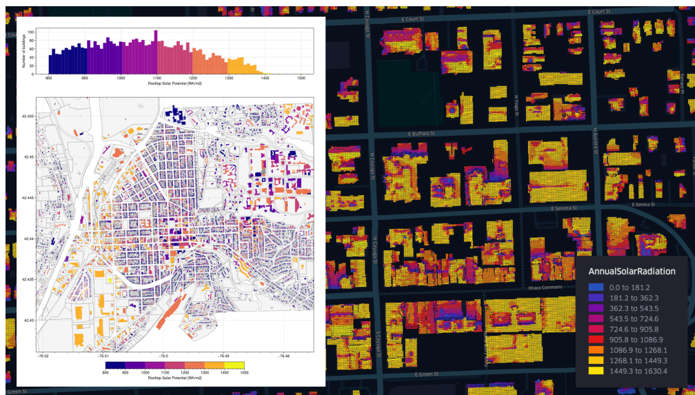
Figure 10: Solar potential of rooftops in Ithaca.
