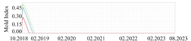
Figure 6 Mold index of the interior surface of the inner concrete layer. Cellulose (red), Rockwool (blue), Sprayed foam (green), and Fiberglass (cyan).
