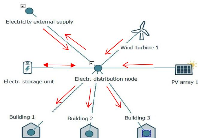
*Figure 3: Network schematic diagram of a electricity distribution network in IES-VPP*
