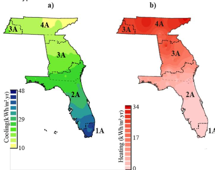
Figure 6 Performance-based maps of a) Cooling and b) Heating energy demand of High-Rise Apartments complying with Zone 1A requirements based on the ASHRAE Standard 90.1-2013.
