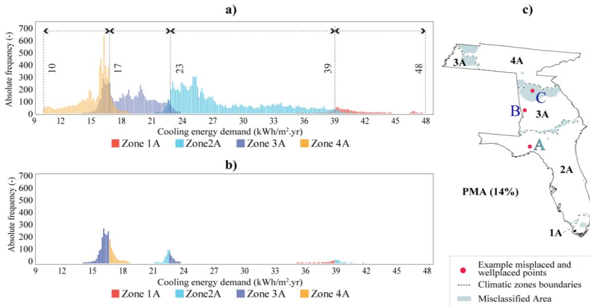
Figure 7 a) Histograms of cooling energy demand for the Zone 1A building b) frequency bars related to misplaced points and c) misplaced areas.
